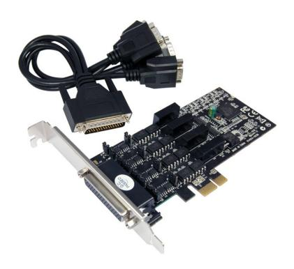
RS-422/485 I/O series, a line of PCI Express Multi-port Serial Communication Board, is designed to meet PCI Express Base Specification 1.1.
