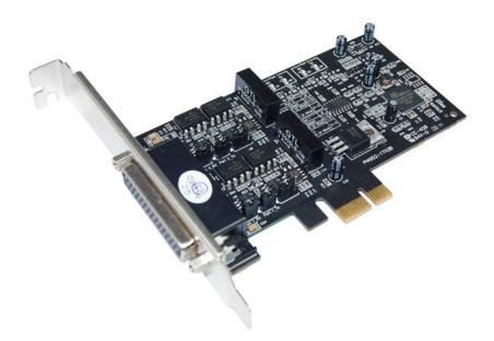
Features Compliant with PCI Express Base Specification 1.1 Supports x1, x4, x8, x16 (lane) PCI Express Bus connector keys Built-in 16C950 compatible UART 128-bype deep transmit/receive FIFOs Serial communication speeds up to 1Mbps RS-422 and RS-485 auto detect and switching Low profile form factor ±15KV ESD protection on all signal pins 2KV isolation protection for all signal and power (Isolation version only) Plug-n-Play, I/O address and IRQ assigned by BIOS
