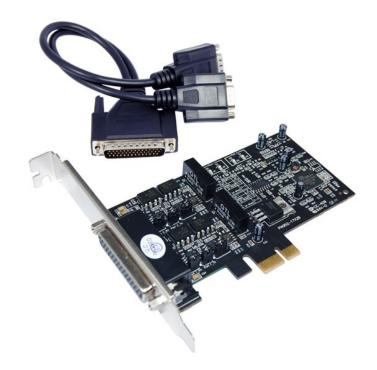
RS-422/485 I/O series, a line of PCI Express Multi-port Serial Communication Board, is designed to meet PCI Express Base Specification 1.1.
