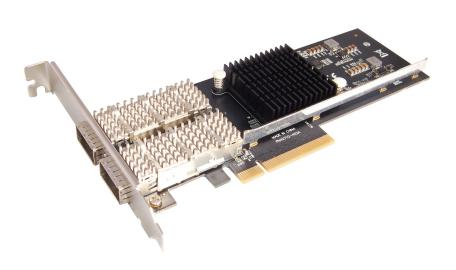
Get fast, high-bandwidth connectivity with this dual-port QSFP+ Network Interface Card. It connect QSFP+ slots to your server or workstation.
