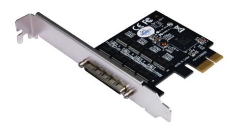
RS-232 I/O series, a line of PCI Express Multi-port Serial Communication Board, is designed to meet PCI Express Base Specification V2.0. It can be installed in virtually any available PC system and compatible with all major operating systems. Users do not need to manually set jumpers to configure I/O addresses and IRQ locations.
